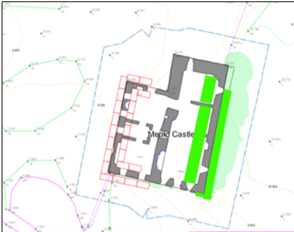
Fig. 3: Plan of structure indicating area of monitoring for scaffolding (red) and area where stone retrieved (green).
